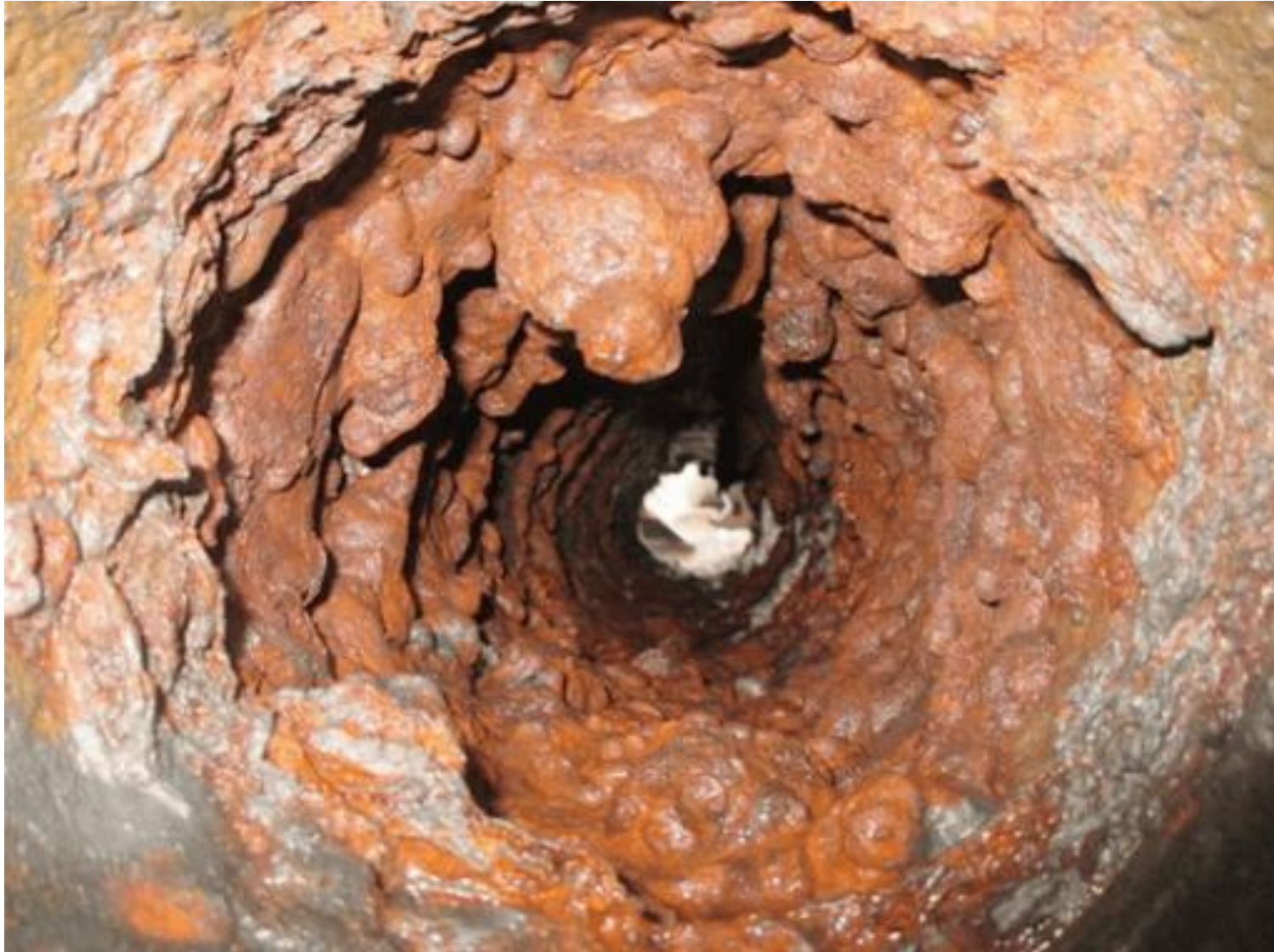
Example of tuberculation in old cast iron pipe.
